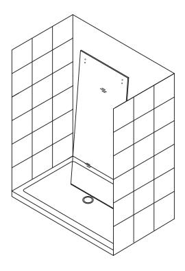
Thoughly clean the edge of the fixed panel. Install the U-Gasket on the fixed panel.
