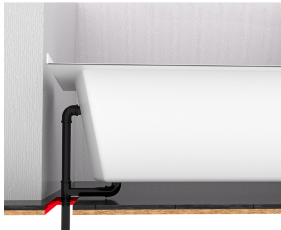
ABOVE THE FLOOR ROUGH-IN INSTALLATION
