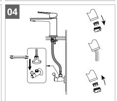
Attach the water lines to your main water supply lines. Ensure that you are connecting the hot and cold lines appropriately. Remove the aerator. Run water and check for leaks. Reinstall the aerator
