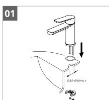
Make sure there is a 35mm-40mm hole on the basin before installing the faucet, Unscrew the fitting ASSY from the bottom of the body, then pass the body through the hole, don't forget to fix the o-ring between the bottom of the faucet and the basin.
