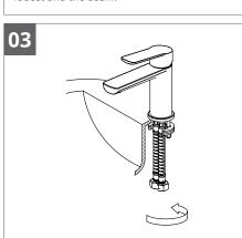
Hand tighten the nuts on the mounting ring provided.
