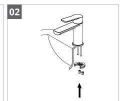
Install the gasket and bracket. Secure the faucet with the nut provided.
