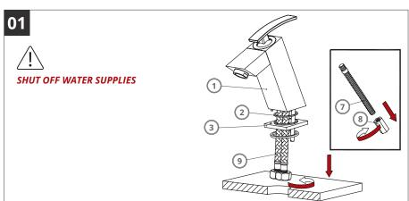
Make a hole of Ø32~35mm on the basin deck, screw of the nut (8) from the long rod (7), screw the long rod (7) and the inlet pipe (9) onto the main body (1), put the main body into the hole with the washer (2), the base (3) and the washer (4) between basin deck and the main body.
