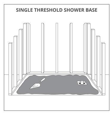
Make sure to apply enough mortar to cover the frame underneath the shower base.
