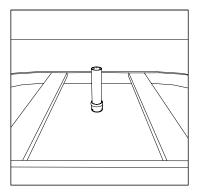
Once the tailpiece is been installed on the waste & overlow, position the Tub and tailpiece in-line with the drain.
