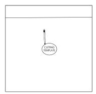
02 Cut 6-1/2" (16.5mm) hole into the wood sub-floor for the drain flange.
