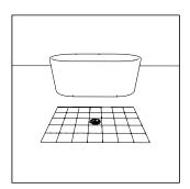
Carefully lower the tub with the installed brass tailpiece as vertical as possible into the red collar in drain assembly.
