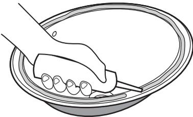
Step 4: Generously apply 100% silicone sealant. Do not use adhesives or adhesive sealants
