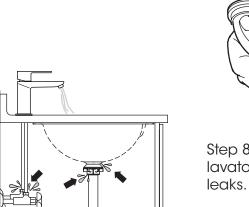
Step 8: Run Water into the lavatory and check for leaks.
