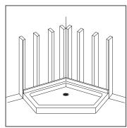
Using a pencil, mark the shower base flange where the wall studs are.
