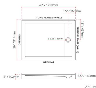
SDTLD4836L1 (LEFT HAND DRAIN LOCATION) (RIGHT HAND THRESHOLD / OPENING)
