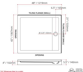
Valley's double threshold, offset linear drain acrylic shower bases are meant to be installed in a corner setting. A white drain cover is included. Complies with CSA & IAPMO standards.
