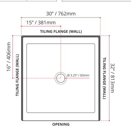
4.5" / 114mm 3" / 76mm DISCLAIMER: Measurements may vary ± ¼" (Diagram Not to scale)
