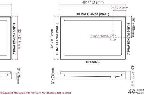
(LEFT HAND DRAIN LOCATION) 48" / 1219mm 9" / 229mm **TILING FLANGE (WALL)** 16" / 406mm TILING FLANGE (WALL) **TILING FLANGE (WALL)** 32" / 813mm Ø 3.25" / 83mm OPENING 4.5" / 114mm / 76mm
