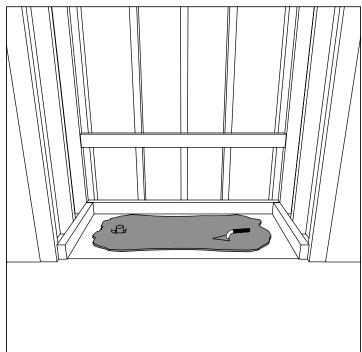
Lift the tub into position. Make sure to align the drain with the pipe. Adjust bathtub legs for leveling purposes.
