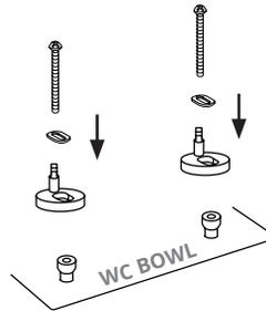
Fit the adjustment plate into the hinge, then place the screw through this assembly.
