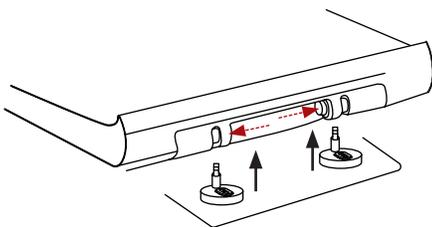
Separate and remove seat from pan. To remove the seat, push both buttons on the seat and lift upwards.
