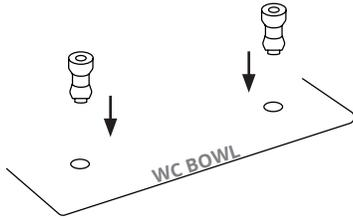
Place the expanding plugs into seat fixing holes.
