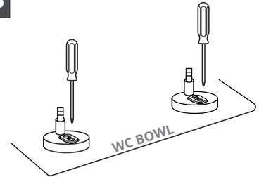
Bolt adjustment plate to the hinge, do not fully tighten - it should still be adjustable.
