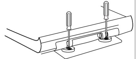
After desire adjustment. Close the seat and lid, then tighten bolts.
