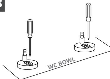
Ensure bolts are fully tightened
