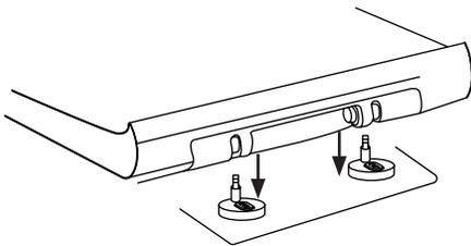
Locate seat hinge over pins and press down until seat "clicks" into place
