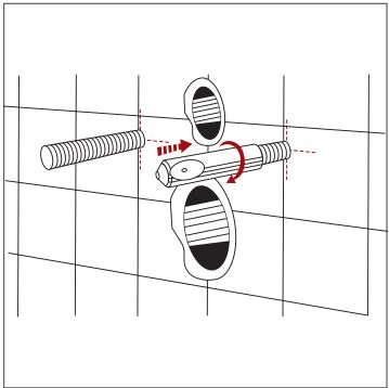
11 Put part **C** into the installing hole on the pan
