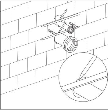
Apply lubricant on rubber washers of the straight tube and connecting pipe, then insert into the ceramic holes as shown.
