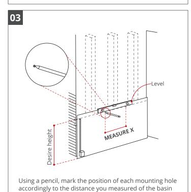
mounting holes. Make sure the mark position is level.
