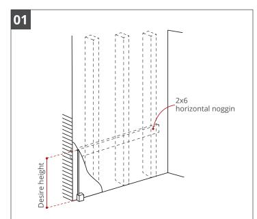
Measure the desire height of the basin and install a 2x6 horizontal noggin.  $\label{eq:contact}$
